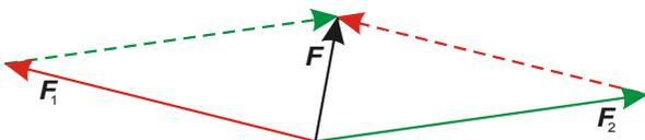
Fig. 1: Vector sum of forces (parallelogram of forces)
