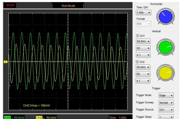
Fig. 9: Oscillation components for a string pendulum describing a circle
