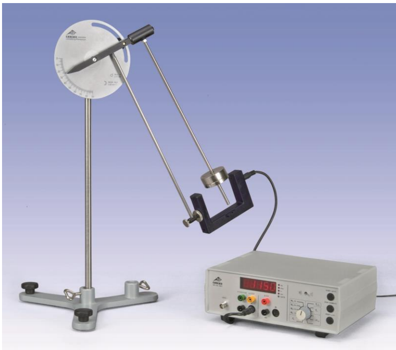
Fig. 1: Variable-g pendulum (photograph and schematic diagram)
