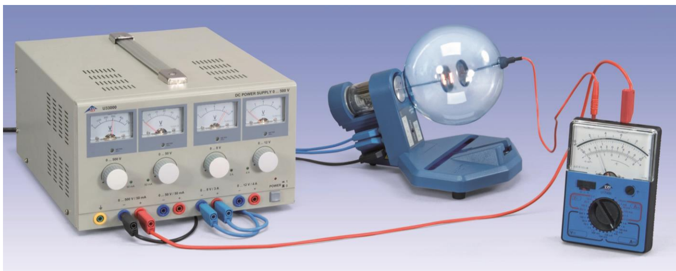
Fig. 1: Circuit (above) and experiment set-up (below) for recording the characteristic of a thermionic diode for different cathode heater voltages (1) Cathode, (2) Anode
